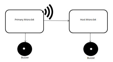
As shown in fig. 5.1, The primary Micro:bit is the main hardware component as it has 3 tasks First it is a processor, secondly it works like a gesture sensor, and it is a radio transmitter.
